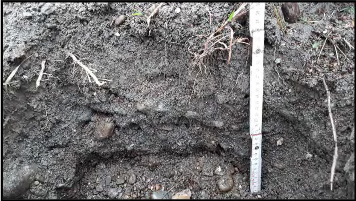
**Plate 38. ST2 within STA4; coarse fill materials from residential development (N/A).**
