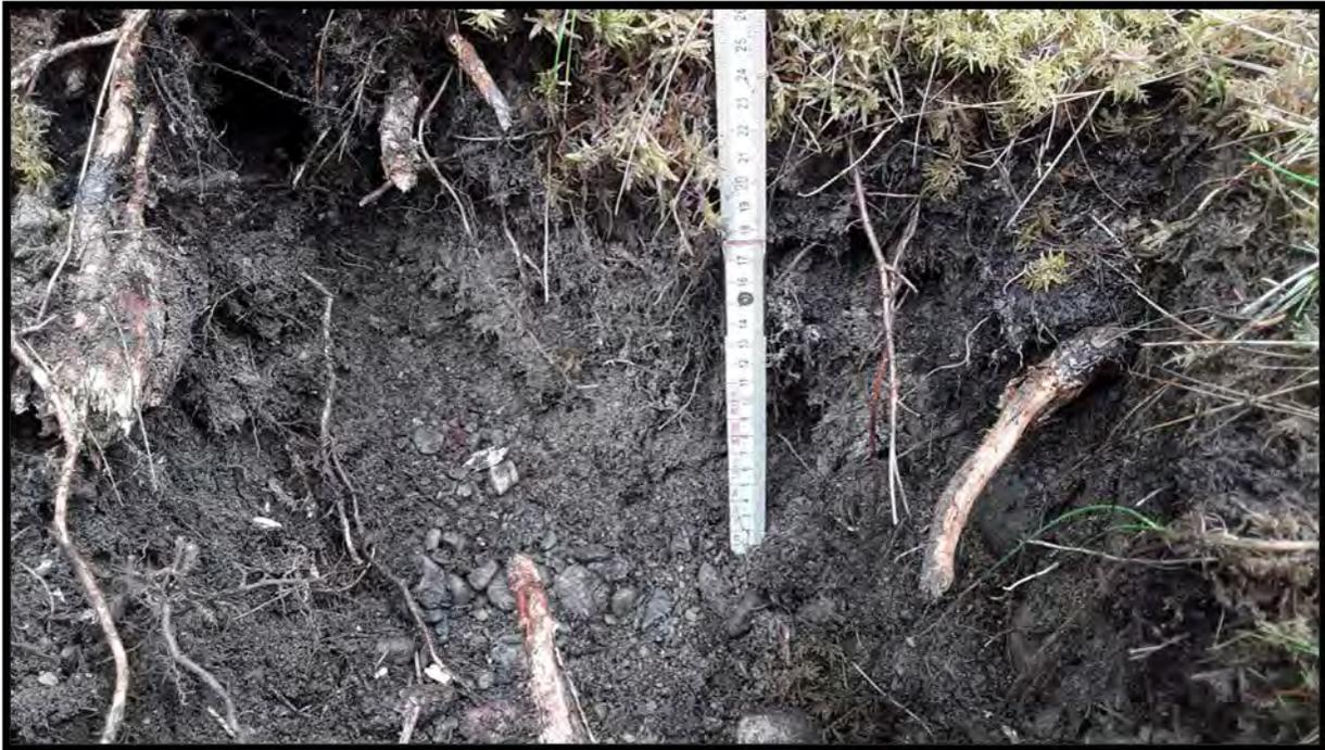
**Plate 34. ST14 within STA3; coarse loamy sand (N/A).**
