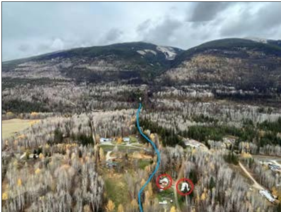
Photo 9: View of Rainbow Creek fluvial fan. A barn (circled, left) and the residence (circled, right) at 385 Koeneman Road are located close to the creek channel. The blue line is the trace of Rainbow Creek.
