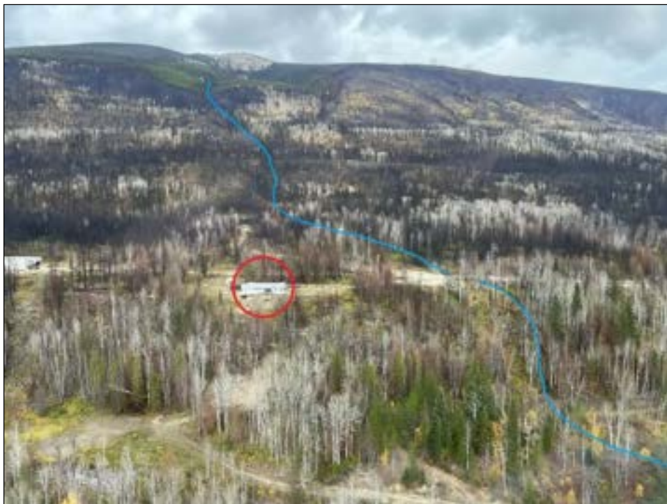
Photo 17: View of the residence at 3100 McBride Highway 16 E (circled) on the north side of Hagan Creek. The creek channel crosses an upper road (not visible) and the HG Road through culverts. The creek has the potential to avulse and be diverted towards the residence.
