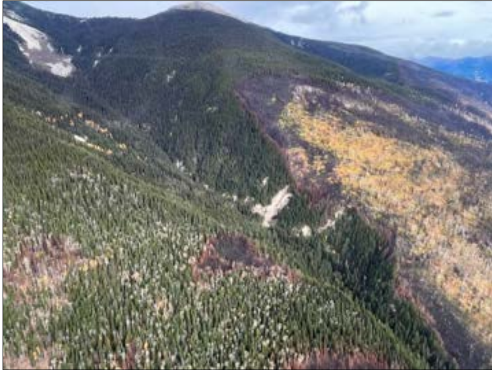
Photo 13: View of the upper end of Face Unit 2 with the large, shallow landslide outlined with exposed light brown bedrock in the headscarp at right centre on the open slope. Rainbow Creek, in the foreground, has several pre-existing, side-slope landslides leading into the main valley.
