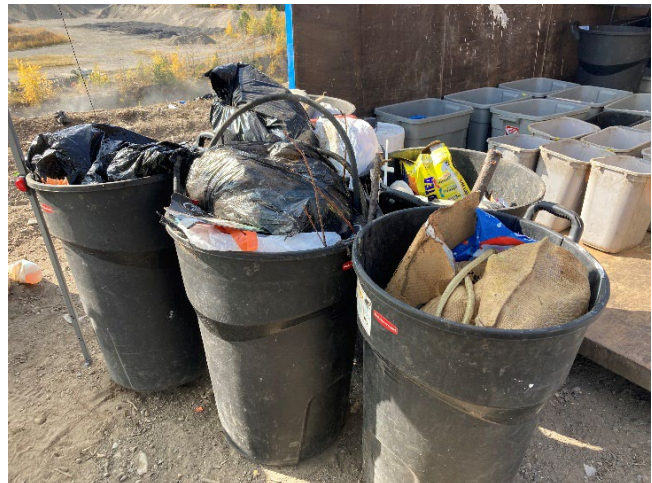
Figure 2-2: 100kg SF Sample to be Hand Sorted
