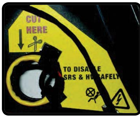
Cut SRS / HV Disable Loop Cable
