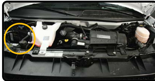
Disconnect the 12V Battery Cables
