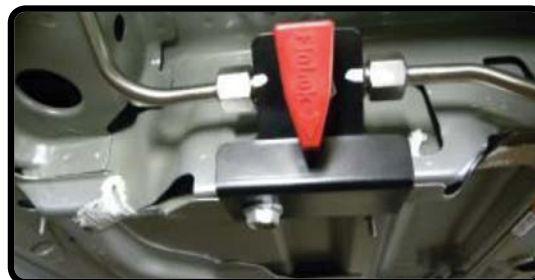
1/4 Turn Shut-Off Valve, Off Points Down
