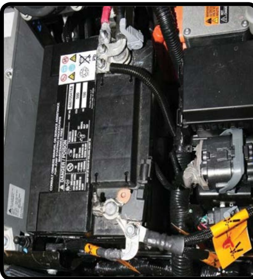
12V Battery Disconnect
