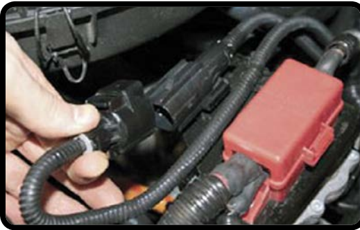
12V Battery Disconnect
