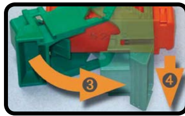
3. Rotate Lever 4. Pull Out Plug
