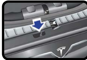
Secondary Hood Catch
