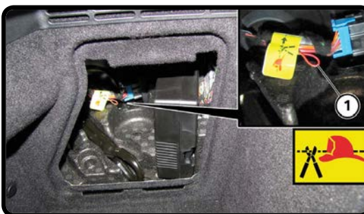
Alternate HV Disconnect Cutting Solution
