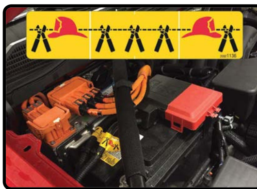
Cut All Marked Low Voltage Cables
