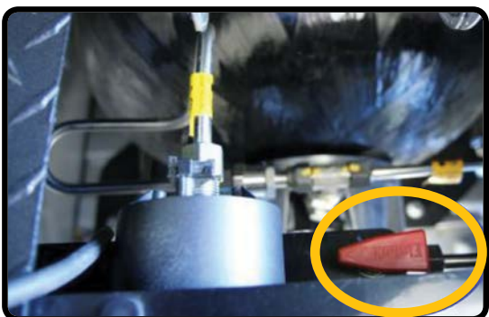
Turn Isolation Valve Counter Clockwise
