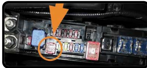
Remove Fuse F/L V IGCT RLY (red)
