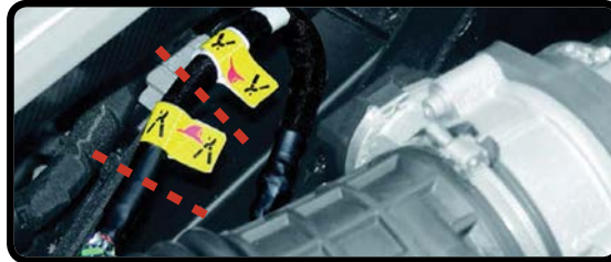
Cut 12V Battery Negative Cable As Marked
