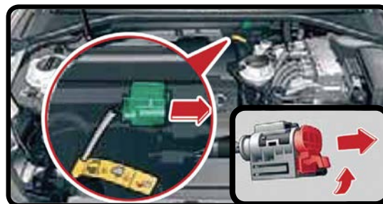
Disconnect HV Emergency Disconnect
