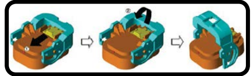
1. Unlock, 2. Release, 3. Remove
