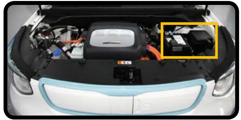
Fuse Box and Battery Location
