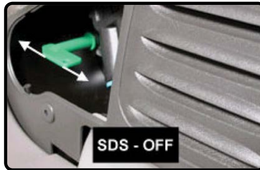
Service Disconnect Switch
