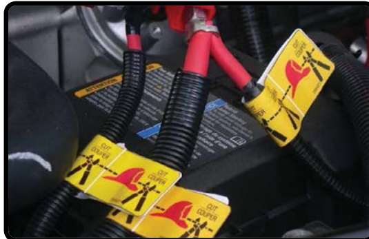
Cut 3 Exposed Cables (Alternate Procedure)
