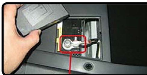
12V Battery Negative Cable In Trunk
