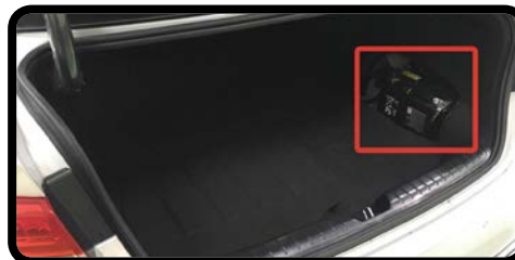
12V Battery Negative Cable in Trunk
