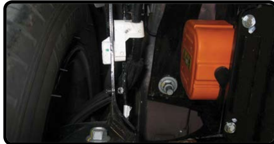
Remove Lower Service Disconnect Fully
