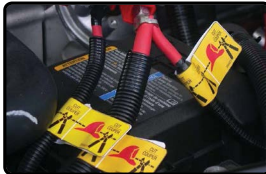
Cut 3 Exposed Cables (Alternate Procedure)
