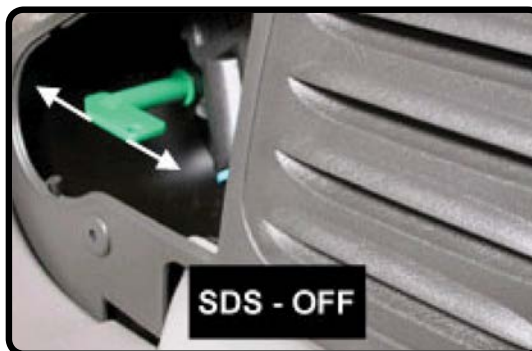
Service Disconnect Switch
