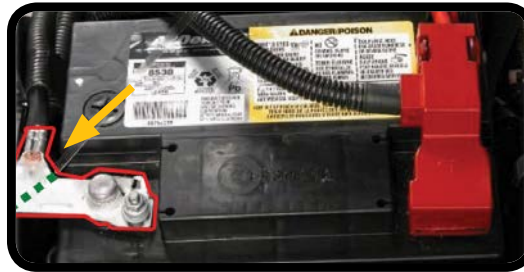
Cut here to disable BOTH 12V negative cables at once.
