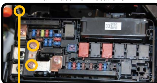
Cut Cable and Main Fuse Screw Locations
