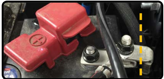
Cut the Positive Battery Cable
