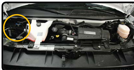
Disconnect the 12V Battery Cables
