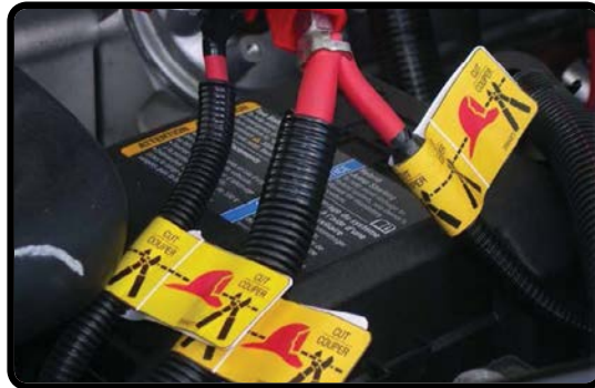
Cut 3 Exposed Cables (Alternate Procedure)
