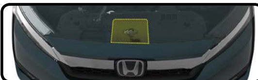
If You Need to Cut The Hood To Open It, Be Sure To Stay Within The Cut Zone
