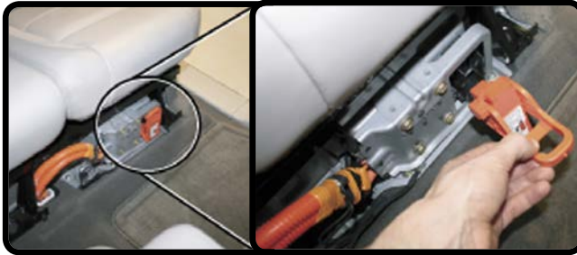
HV System Disconnect
