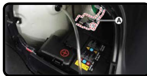
12V Battery Negative Cable
