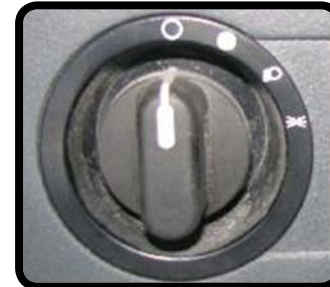
Power Switch Off Position
