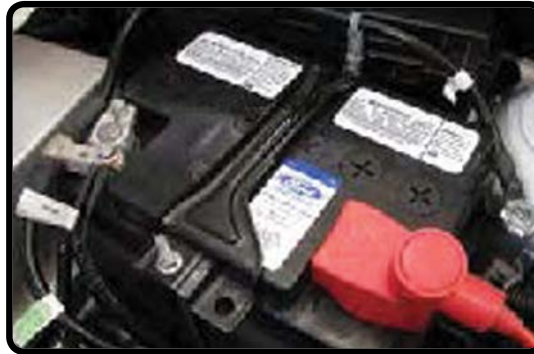
Disconnect 12V Battery Negative Cable in Engine Compartment on Driver's Side
