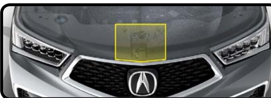
If You Need to Cut The Hood To Open It, Be Sure To Stay Within The Cut Zone
