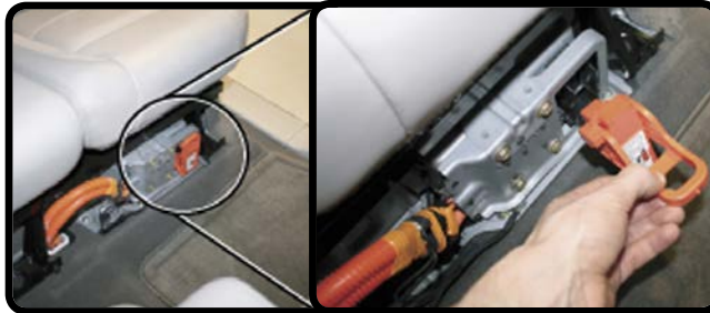
HV System Disconnect
