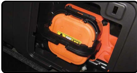
Remove Upper Service Disconnect Fully
