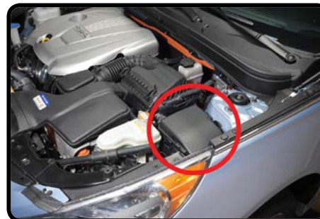
Fuse Box Location
