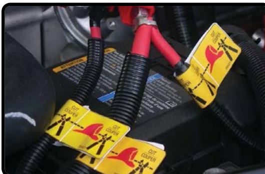
Cut 3 Exposed Cables (Alternate Procedure)
