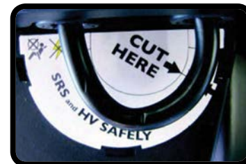
Cut SRS / HV Disable Loop
