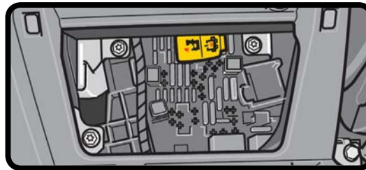
Fuse Box Location
