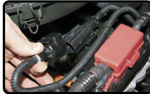
12V Battery Disconnect
