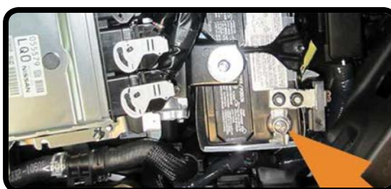
12V Negative Disconnect Under Hood
