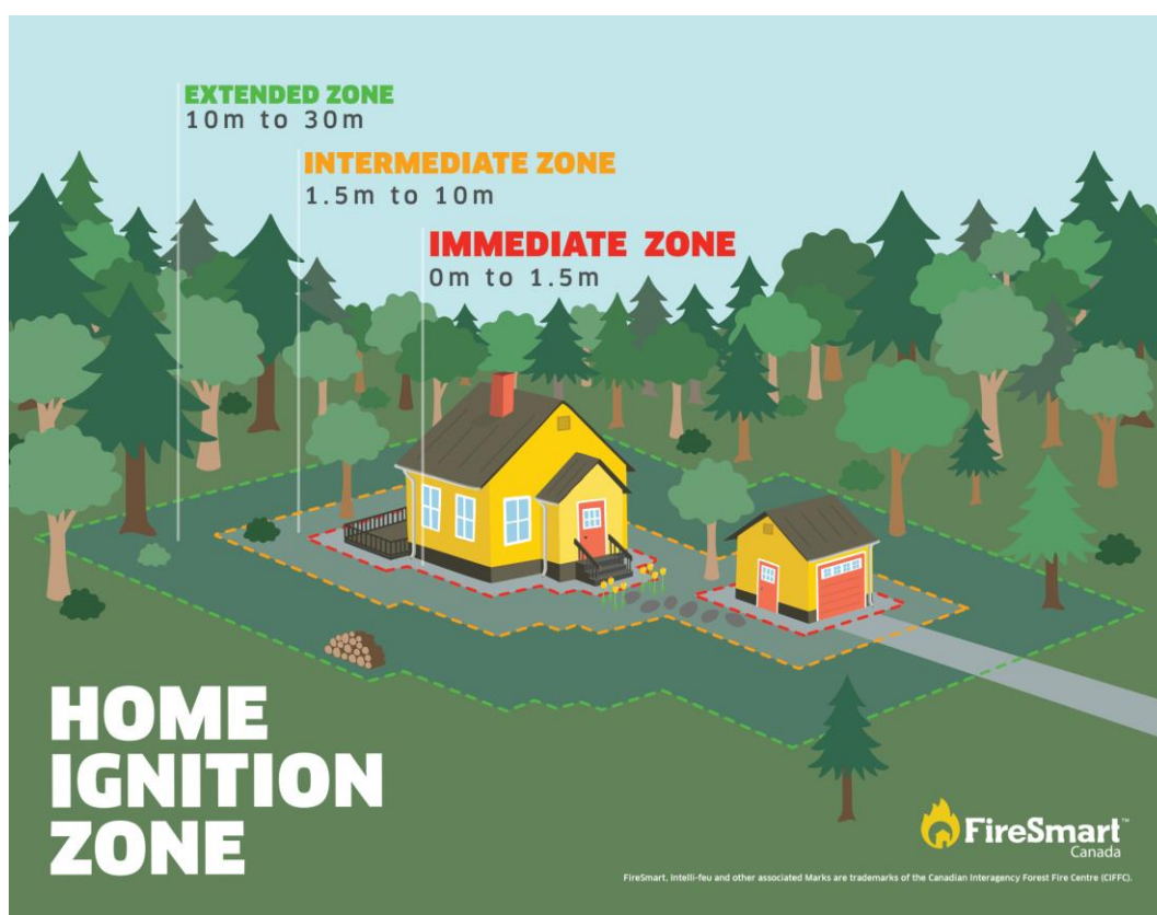
Figure 16. FireSmart Home Ignition Zone, which is comprised of four priority zones, as illustrated in the BC FireSmart Begins at Home Manual
